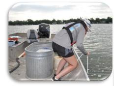
it into the turbidity meter. A light shines through the water sample. The light beam is scattered by the suspended solids which measures how clear the sample is. A dissolved oxygen meter is used to take the dissolved oxygen levels just below the water surface.
